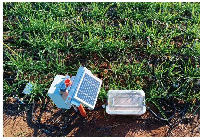
Left to right: Logger, solar panel and wiring junction box for soil water content and matric potential sensors (top right) at Armatree, NSW. June 2024. Photo credit: J. Eberhard, UniSQ
