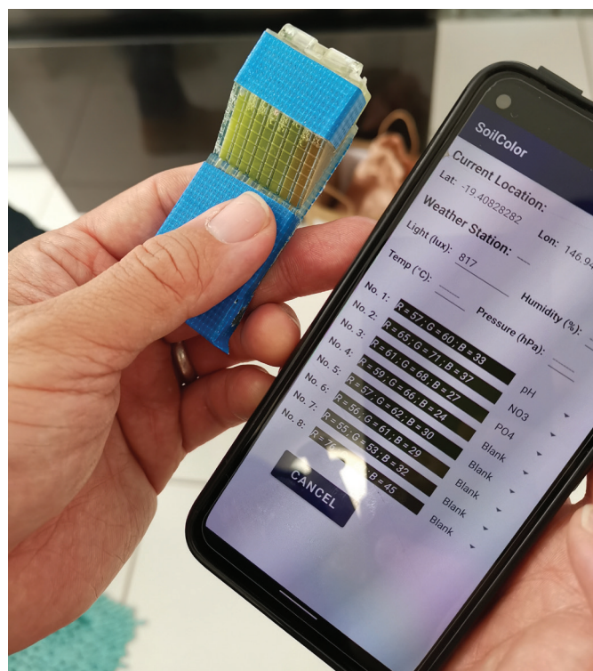
Smartphone app interface demonstrating how the colorimetric test results are displayed.
