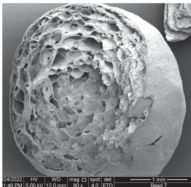
Scanning electron microscope (SEM) images of polymer beads containing clay minerals and loaded with imidacloprid.
