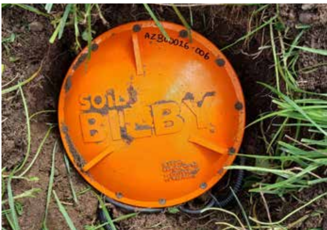
The BILBY® wireless communication node being installed in the field (source: Tasmanian Institute of Agriculture).
