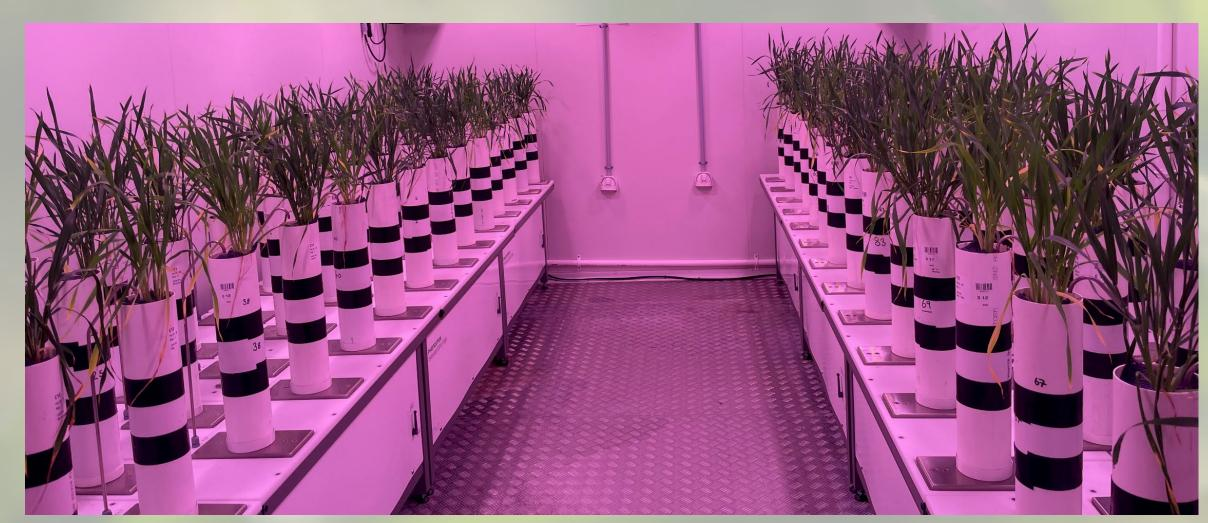
A series of glasshouse experiments use soil from key sites to explore the interplay between soil moisture, strength, and root growth within this hardsetting soil type, and to investigate potential amelioration strategies.
