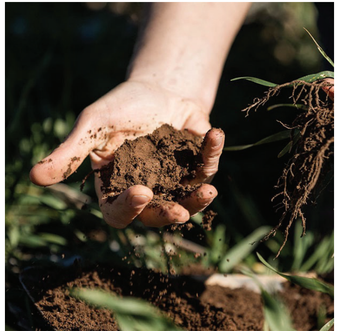
Soil texturing in the field to estimate sand, slit, clay % (Source: Soil CRC)
