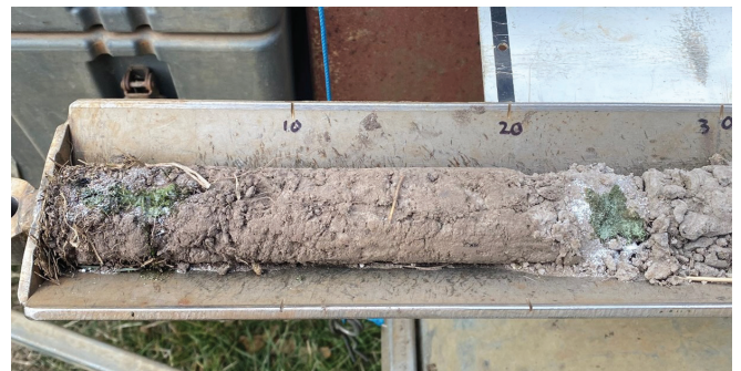
Soil sample 0 to 30cm depth from a pasture paddock (Source: Felicity Harrop)
