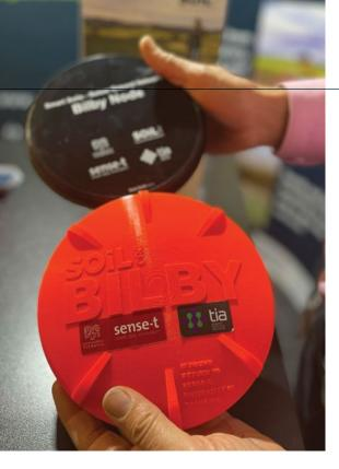
Program 2 researchers are also working to enable easier and safer communication of data from within and under crops and pastures. The Bilby™ is an underground communication node. It can send signals from deep within the soil to above ground networks, making it safe from potential damage by livestock and machinery. It can be linked to a range of soil sensors, such as soil moisture and salinity probes, and soil temperature sensors.
